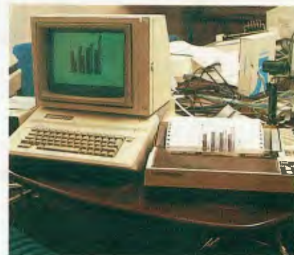
3.15: We thought someone had made a mistake and packed a printer instead of a digitiser. We were wrong. The Apple II Digiscan reads images in through a printer with an interchangeable platen
