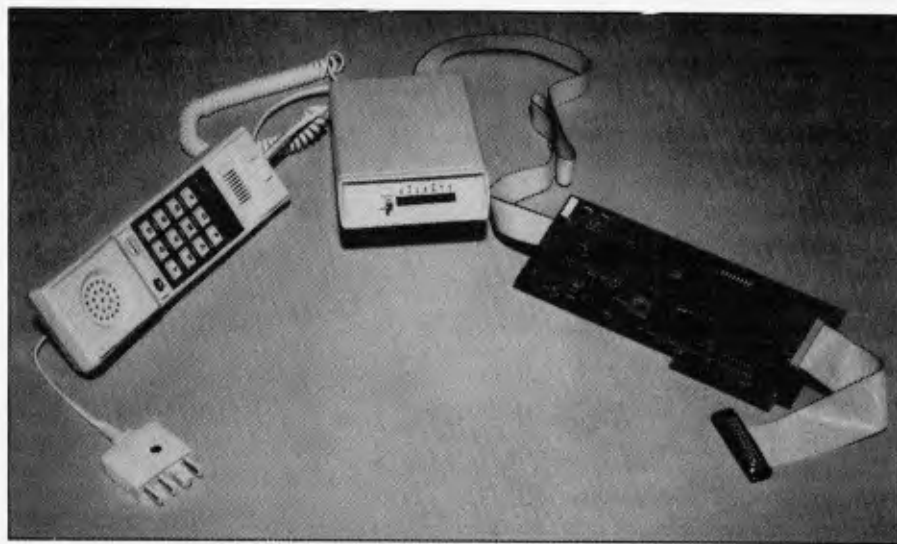
Netcomm Apple Modem cards and software let Apple computers talk to IBM, Prime, Amdahl, DEC, Wang, Facom, Natsemi, Univac, Burroughs, and ICL mainframes
