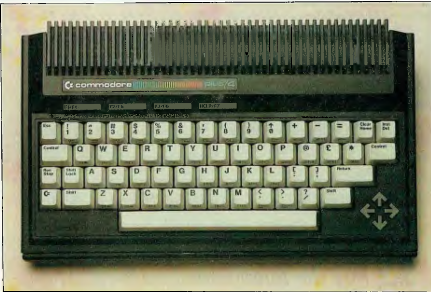
The keyboard features a full qwerty layout and an MSX-style cursor cluster
