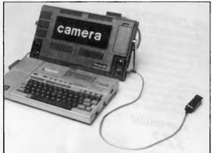
View Scan Text System magnifies text for the partially sighted
